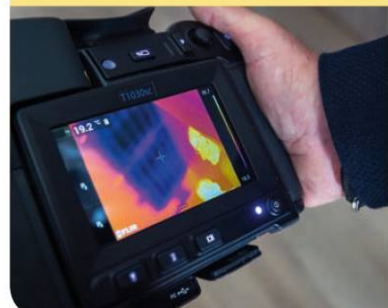
A thermal imaging camera (below) reveals the Radiana system in action behind the ceiling at this luxury London apartment (pictured above)
